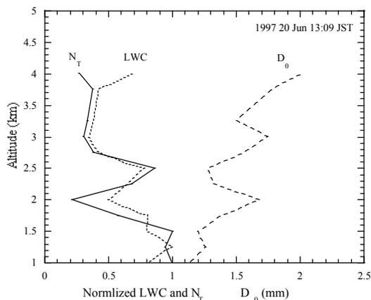
Fig.2 Vertical profiles of LWC,  $D_0$ , and  $N_t$  at 13:09. The Values LWC and  $N_t$  are normalized by the maximum values in the profile. The inverse relation between  $D_0$  and  $N_t$  is clearly seen.
